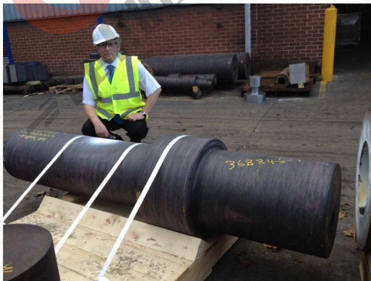
Image 2: A forging for a tubing hanger of alloy 945.
